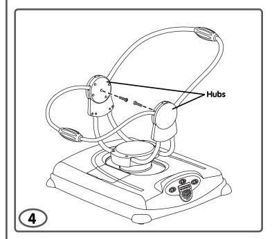
• Insert a #8 x 3,2 cm screw into each hub and tighten.
